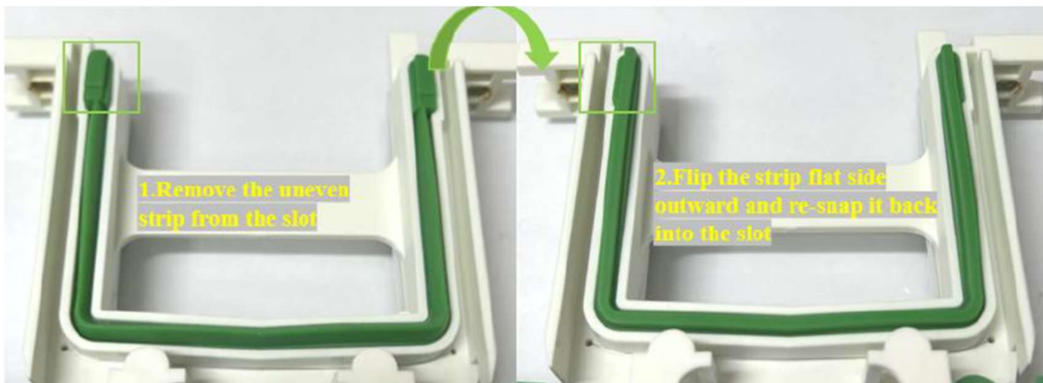
Figure 2. Certain raised electrophoresis tanks may require the silicon seal to be flipped over and resealed in the frame groove with the flat side facing upward.
